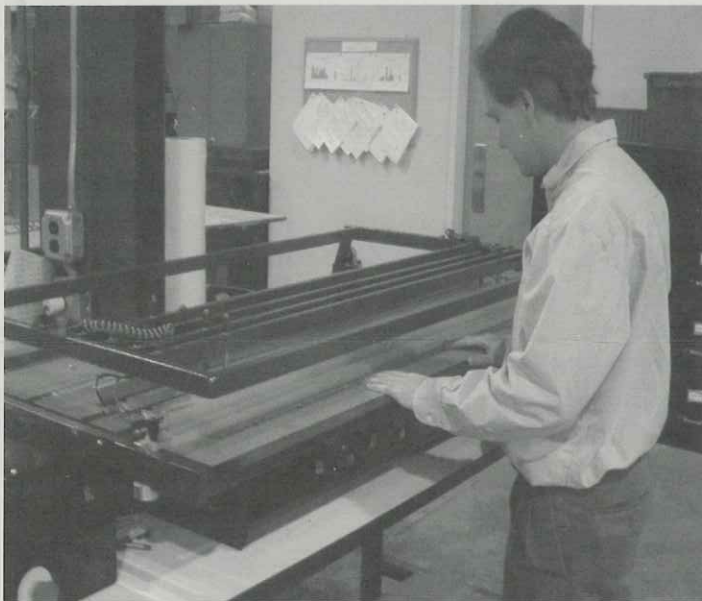
Material is being adjusted by Sean O'Sullivan, Q A Manager, as it is set up to be heated and pressed into shape.
