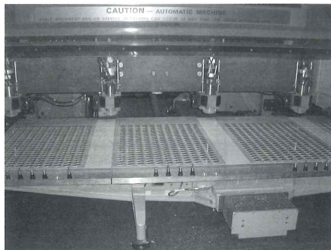
The CNC Drilling and Routing machine can drill holes as small as 0.010" diameter, with tolerances well within 0.005"
