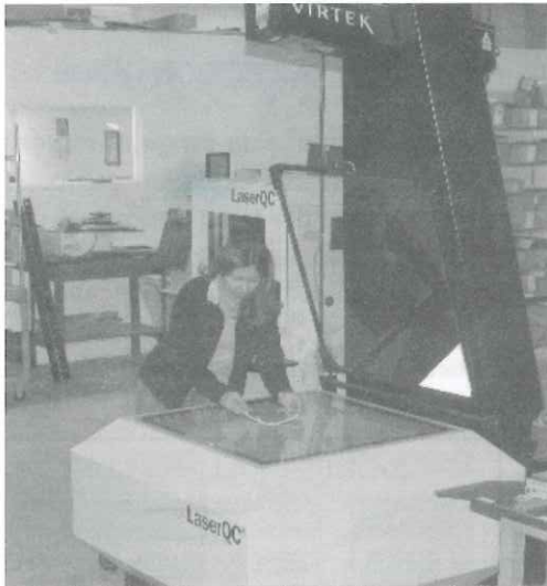
QC Technician Elsy Bedard positions a medical device gasket onto the scanner for accurate comparison to its CAD reference image.
