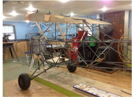
J-3 Piper Cub wing and fuselage assembled
