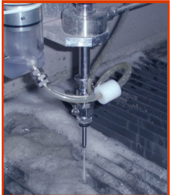
ORION's Waterjet is capable of abrasive & plain water cutting
